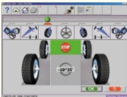
If the operator stops turning the wheel after the basic caster swing, the machine concludes that this is all the operator wants to do and proceeds on to the measurement screen
