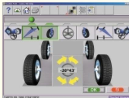
If the operator continues turning the wheel beyond this point, the machine knows that a toe-out-on turns measurement is desired and continues accordingly.
